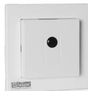
The sensor is designed to detect the presence of a person by motion detection and increase the ventilation demand (70% for 15 minutes). In addition, through a relay, the sensor can switch on the light.
