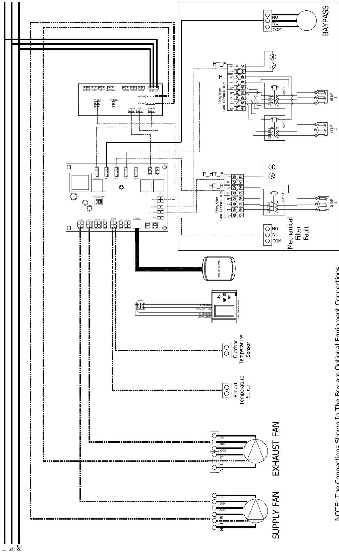
NOTE: The Connections Shown In The Box are Optional Equipment Connections.
