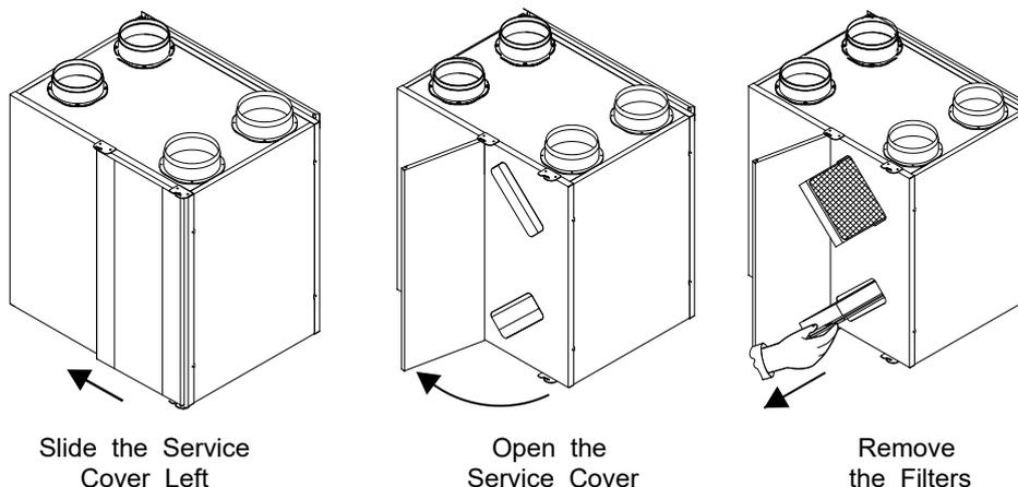
**Step 1:** Slide left, open the service cover and then remove the filters.
