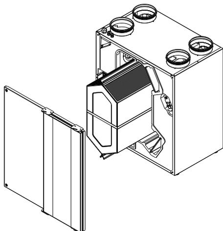
**Step 1:** Remove the front cover plate (see page 8), then remove the by-pass (see page 9) and then remove heat exchanger out from the main unit.
