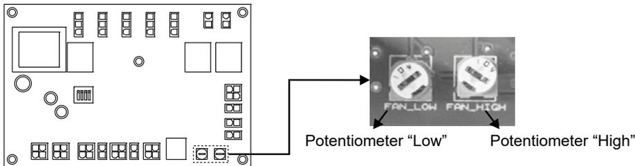
**Note:** If „Low” is set to the highest and „High” is set to the lowest value, unit continues to run according to default settings. Factory setting values can be change.
