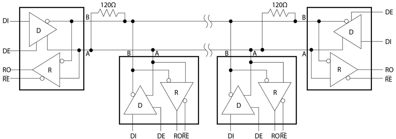
If the line is too long or if any communication problem occurs, 120 Ohm resistance should be added at the beginning and end of the line as shown on schema.
