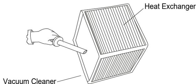
**Step 2:** No cleaning with fluids (including water); only careful dust removal from air intake surfaces with a household vacuum cleaner.
