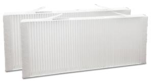
G4 pleated panel filters creates a larger media surface area for air filtration and ensures lower pressure drops. Filters are classified as in the ISO Coarse 70% according to ISO 16890 standards.
